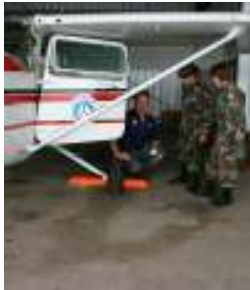
Maj. Norm Morresette walks Cadets Allison and Danielle Greer through a Pre-Flight Inspection of a CAP Aircraft
